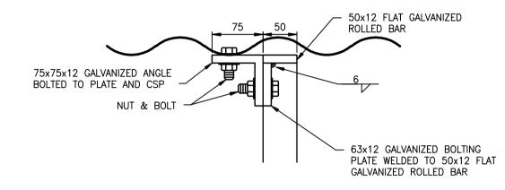
SAFETY GRATE BAR SCREEN — DETAIL SCALE 1:5
