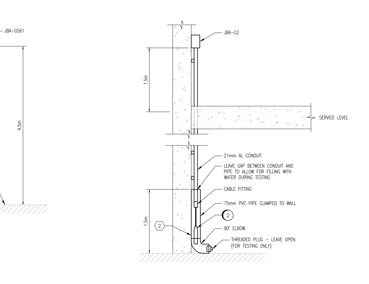
B DRY WELL - FLOOD LEVEL TRANSMITTERS
