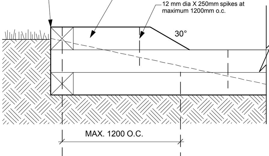
ON SLOPING GROUND, TIMBERS ARE TO REMAIN LEVEL AND ADDITIONAL ROWS ADDED AS REQUIRED.
