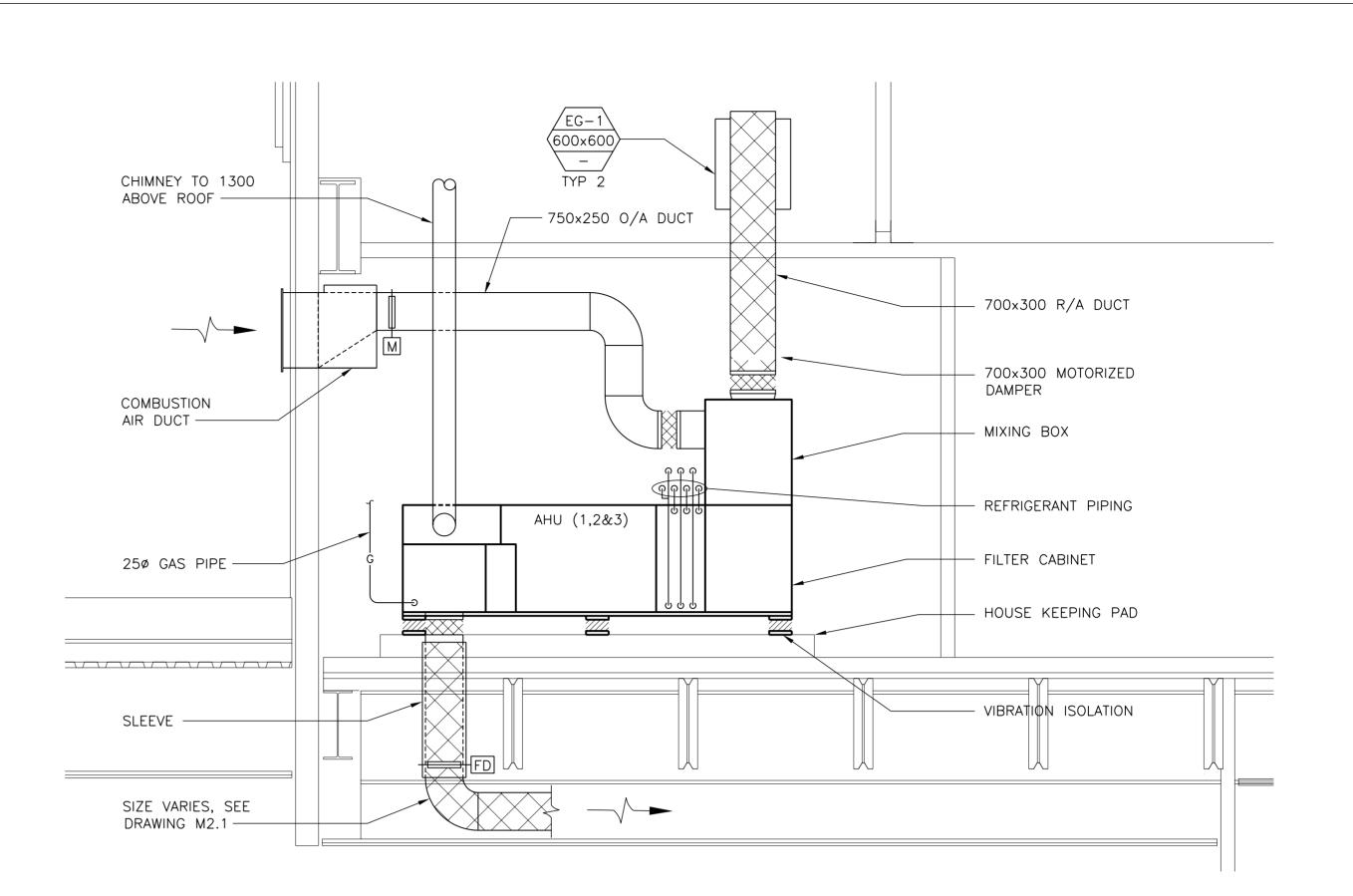
TYPICAL CORNER MECHANICAL ROOM SECTION 1:25
