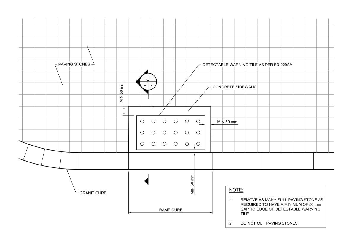
1 DETECTABLE WARNING TILE AT CURB RAMP
