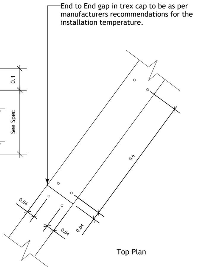
Trex Cap to be predrilled and screwed to Base course using screws. Screws shall be Stainless Steel or Ceramic Coated and approved for use with ACQ treated wood. Screws to extend into timber base a minimum of 5 cm and be countersunk into Trex. Two screws are to be placed at each end and every 60 cm along length. Strait sections of Trex are to be butt jointed.
