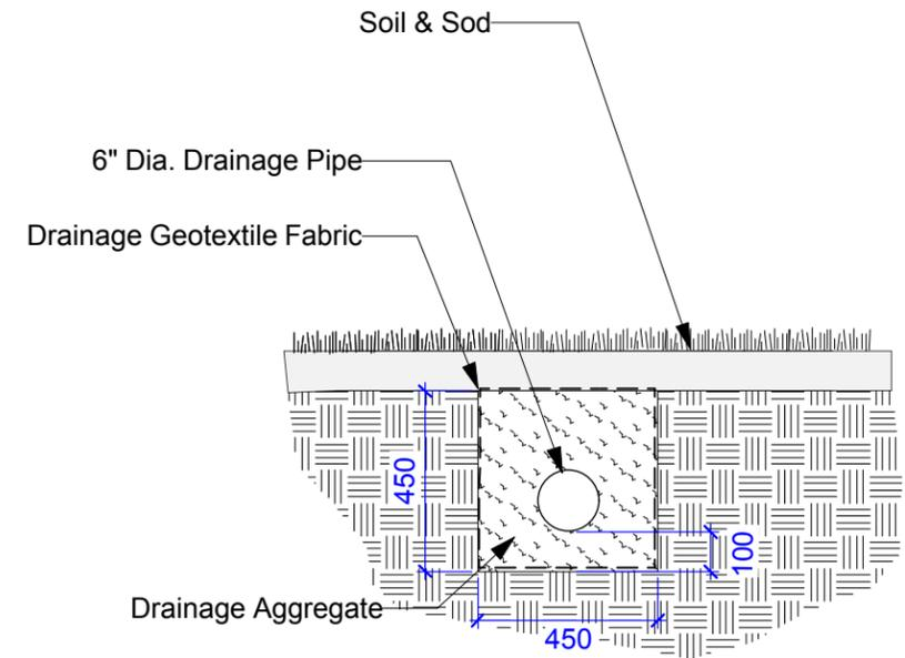
**DRAINAGE CHANNEL TO CATCH PIT DETAIL**
