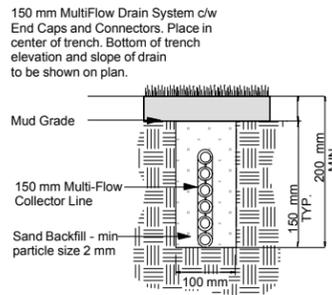
INSTALL MULTI-FLOW IN THE CENTER OF THE TRENCH. BACKFILL MATERIAL SHOULD BE A VERY COARSE SAND. MIN. RECOMMENDED SLOPE 1%.
