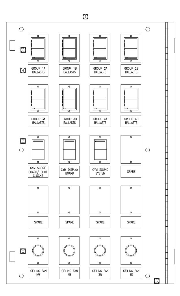
PROVIDE CONDUITS SIZED FOR FOUR 12 GA WIRES PER SWITCH LOCATION.
