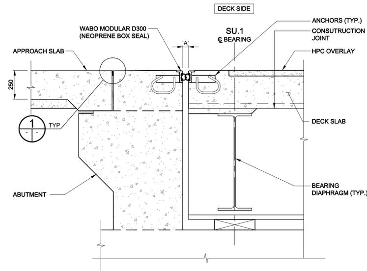
SECTION C SCALE 1:15 (SHOWING EXPANSION UNIT LOOP ANCHORS IN ROADWAY AT SU.1) 40/41
