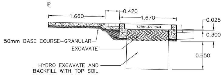
DETAIL "A" - EXCAVATE 50mm BASE COURSE MATERIAL-GRANULAR -HYDRO EXCAVATE AND BACKFILL WITH TOP SOIL
