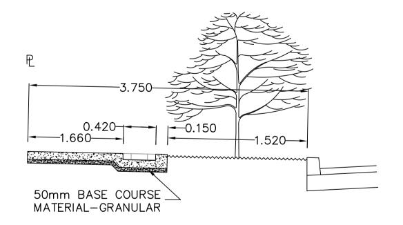
100mm CONCRETE SIDEWALK CROSS SECTION AT TREES
