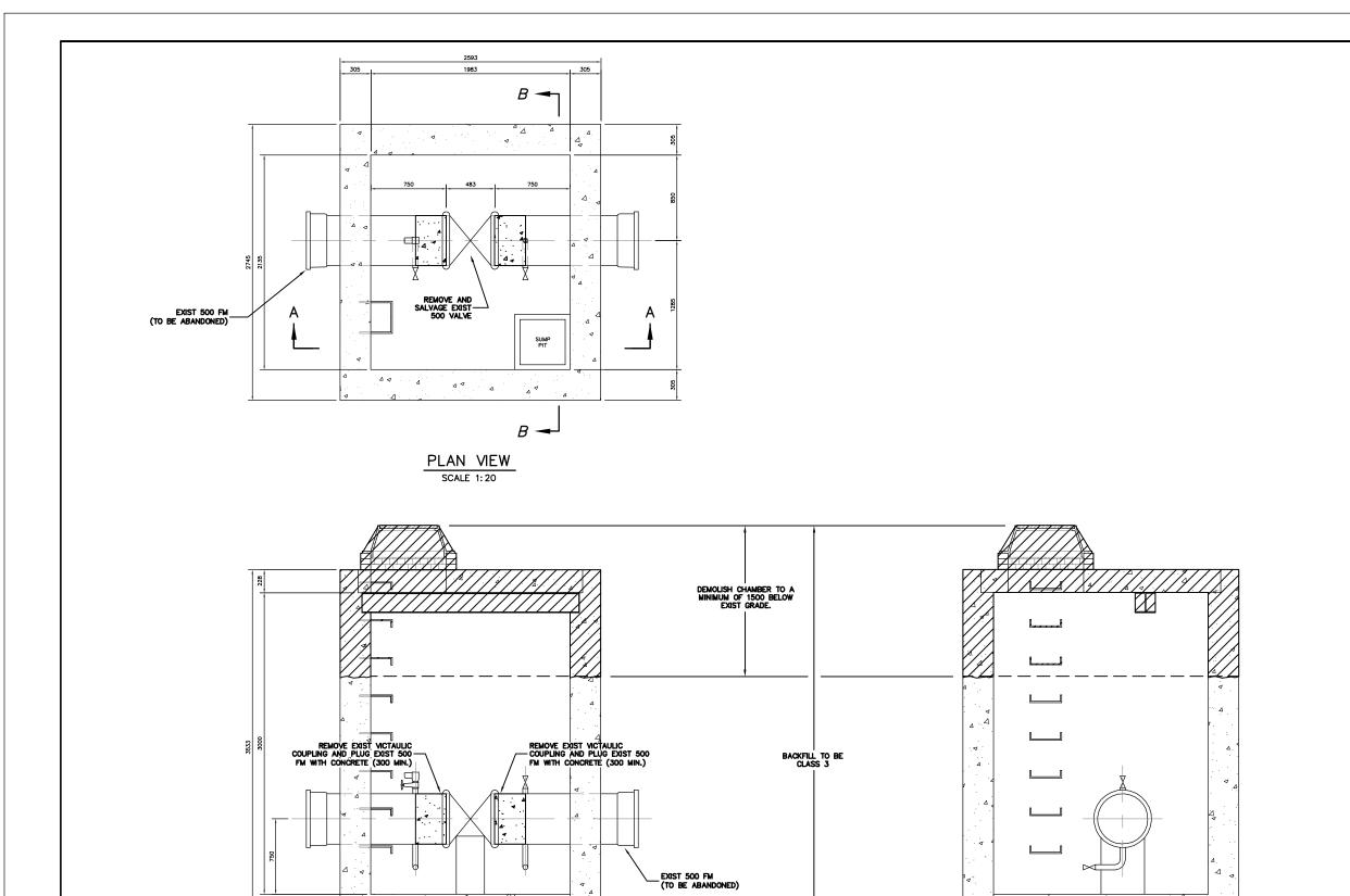
REMOVE SUMP GRATE AND HAND PACK WITH FILL
