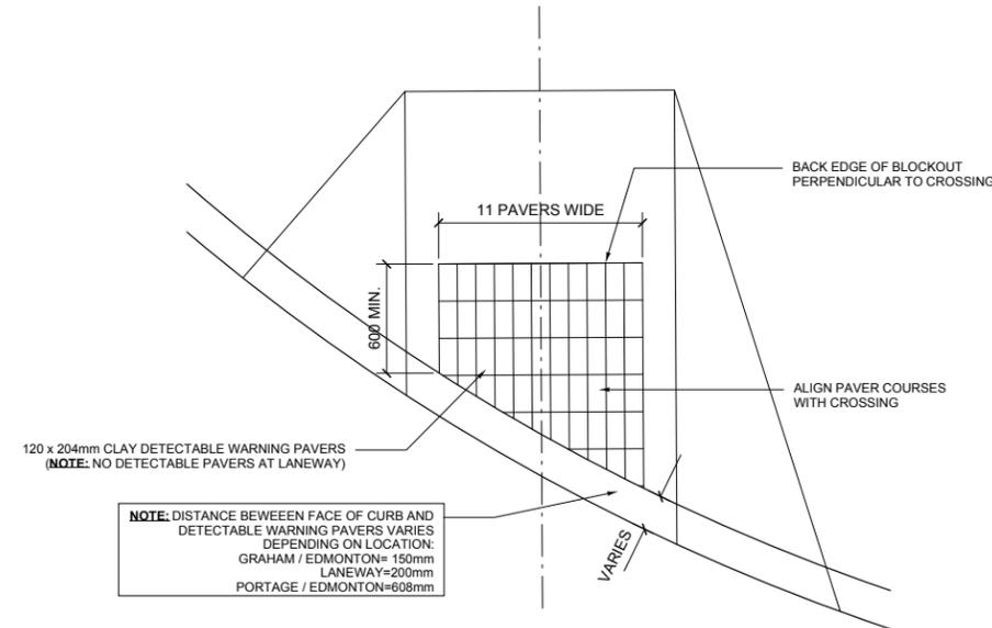
4 DETECTABLE WARNING AT SIDEWALK RAMP (TYP.)
