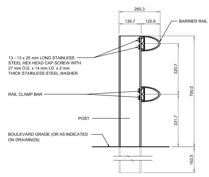
DIMENSIONS FOR HEIGHT OF CENTERLINE OF BARRIER RAILABOVE FINISHED SURFACE AND BETWEEN BARRIER RAILS TO BE CO-ORDINATED WITH POCKET DETAIL FOR CONCRETE TRAFFIC BARRIER.
