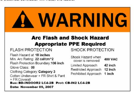
Figure 1 – Example of Arc Flash Warning Label
