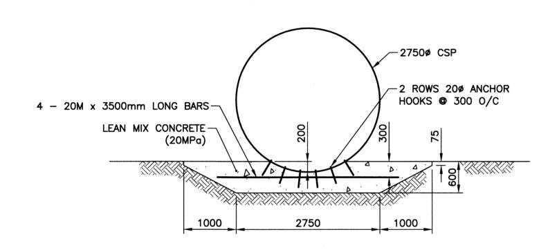
CONCRETE SUPPORT DETAIL SCALE: 1:50
