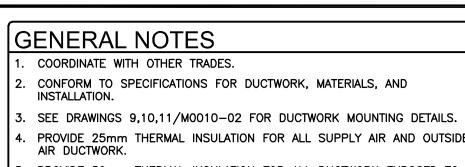
PROVIDE 25mm THERMAL INSULATION FOR ALL SUPPLY AIR AND OUTSIDE
