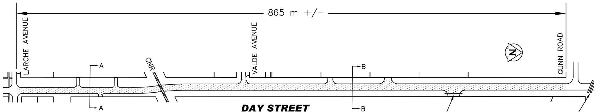
**NOTE:** REMOVE & REPLACE EXISTING 900mm CSP AT #2500 DAY STREET(Approach) WITH 27m - 900mm CSP
