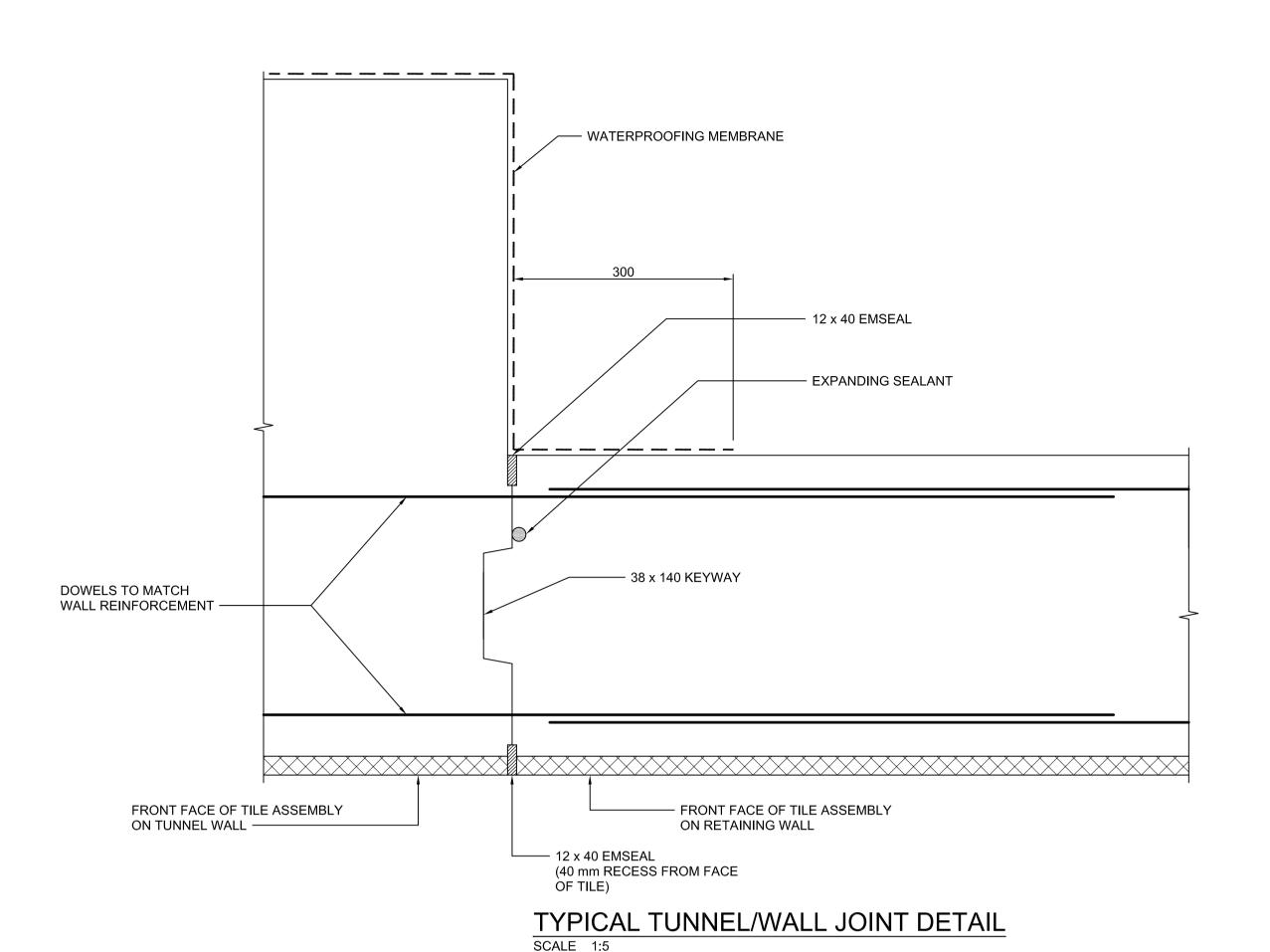
12 x 40 EMSEAL ----— EXPANDING SEALANT REINFORCEMENT CONTINUOUS —— — 38 x 140 KEYWAY FRONT FACE OF TILE ASSEMBLY FRONT FACE —— 12 x 40 EMSEAL (40 mm RECESS FROM FACE OF TILE)
