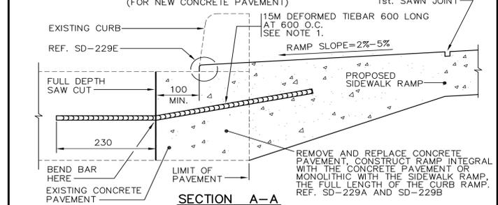
SECTION A-A (FOR EXISTING CONCRETE PAVEMENT)
