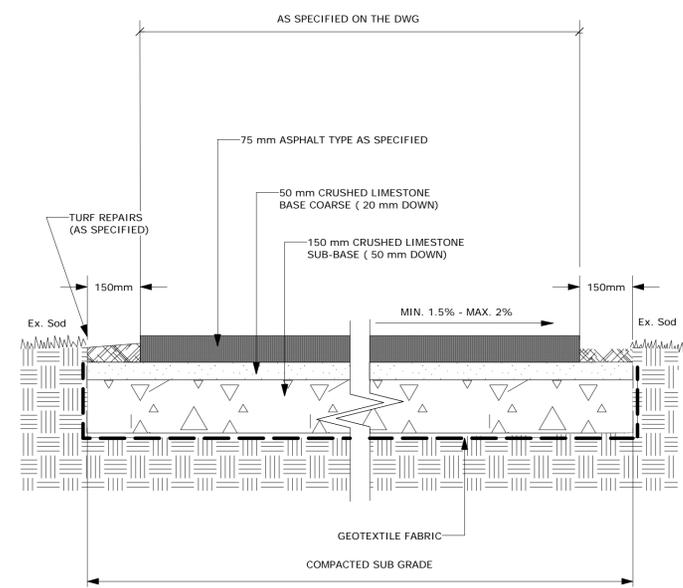
ASPHALT PATHWAY CROSS SECTION
