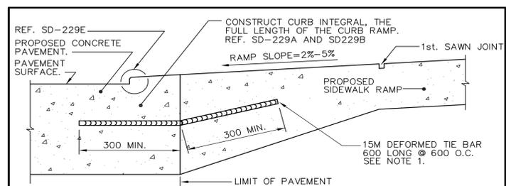
SECTION A-A (FOR NEW CONCRETE PAVEMENT)
