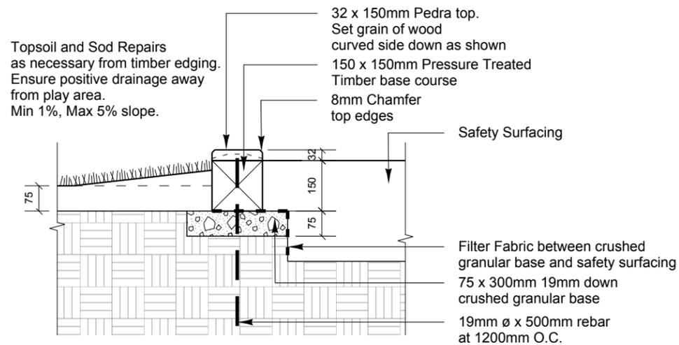
Topsoil and Sod Repairs as necessary from timber edging. Ensure positive drainage away from play area. Min 1%, Max 5% slope.
