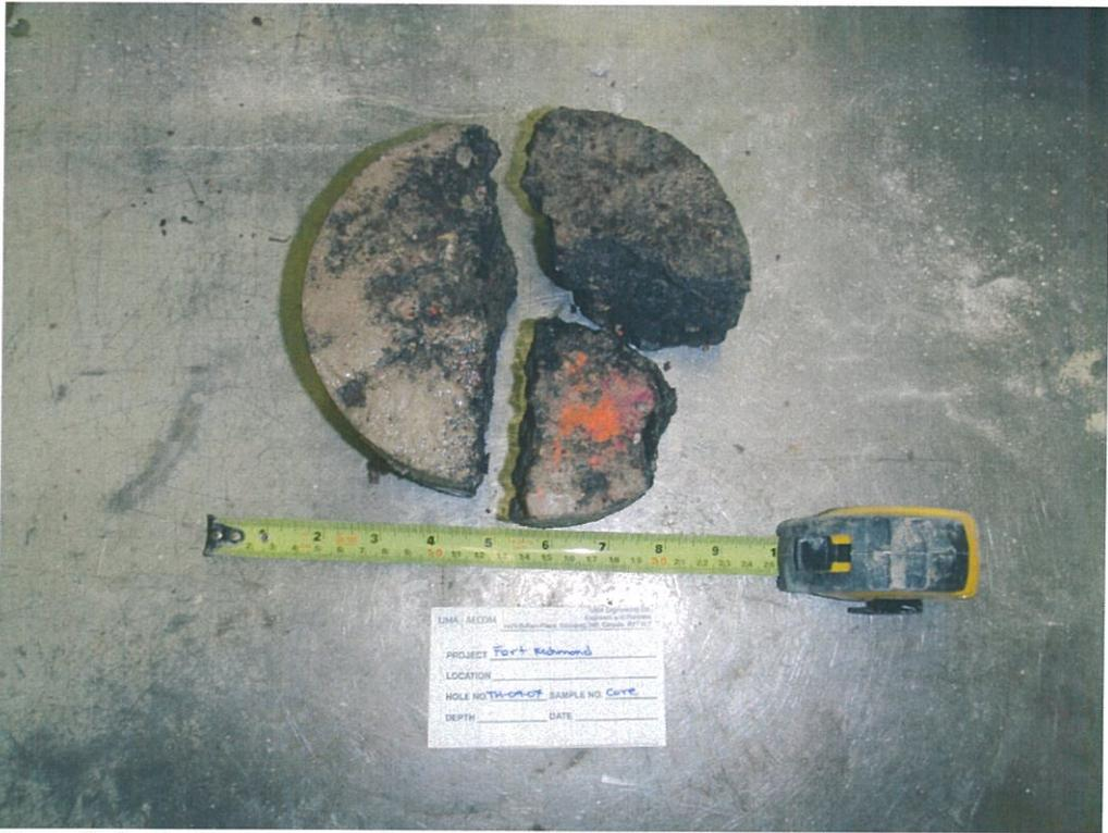
Photo 8: Asphalt core sample from TH-09-07
