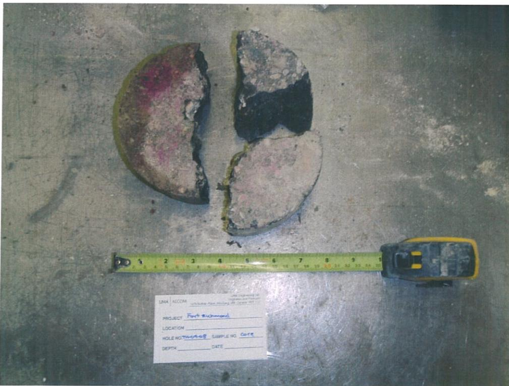
Photo 10: Asphalt core sample from TH-09-08
