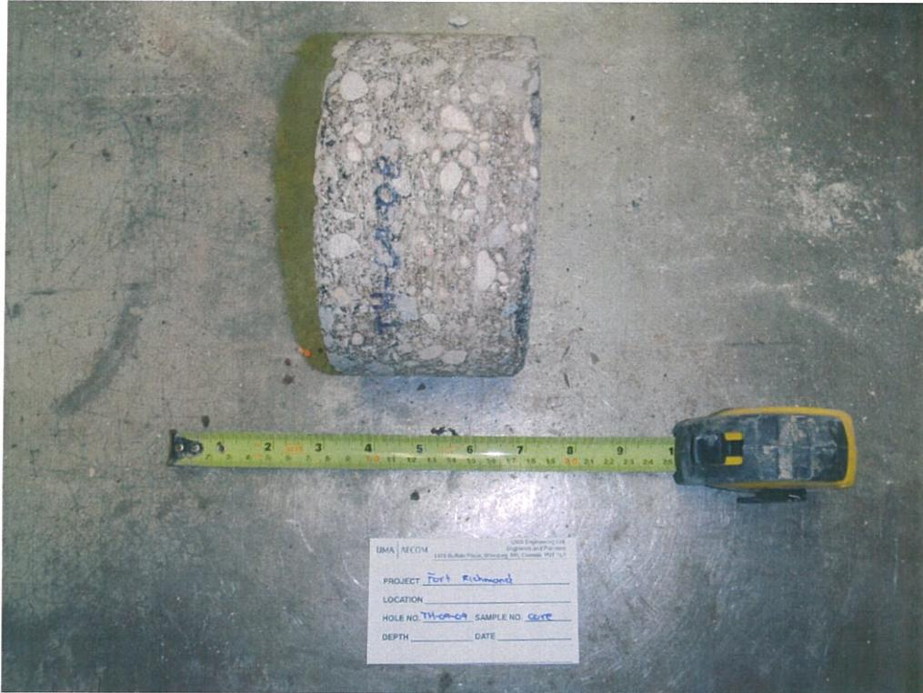
Photo 11: Asphalt core sample from TH-09-09
