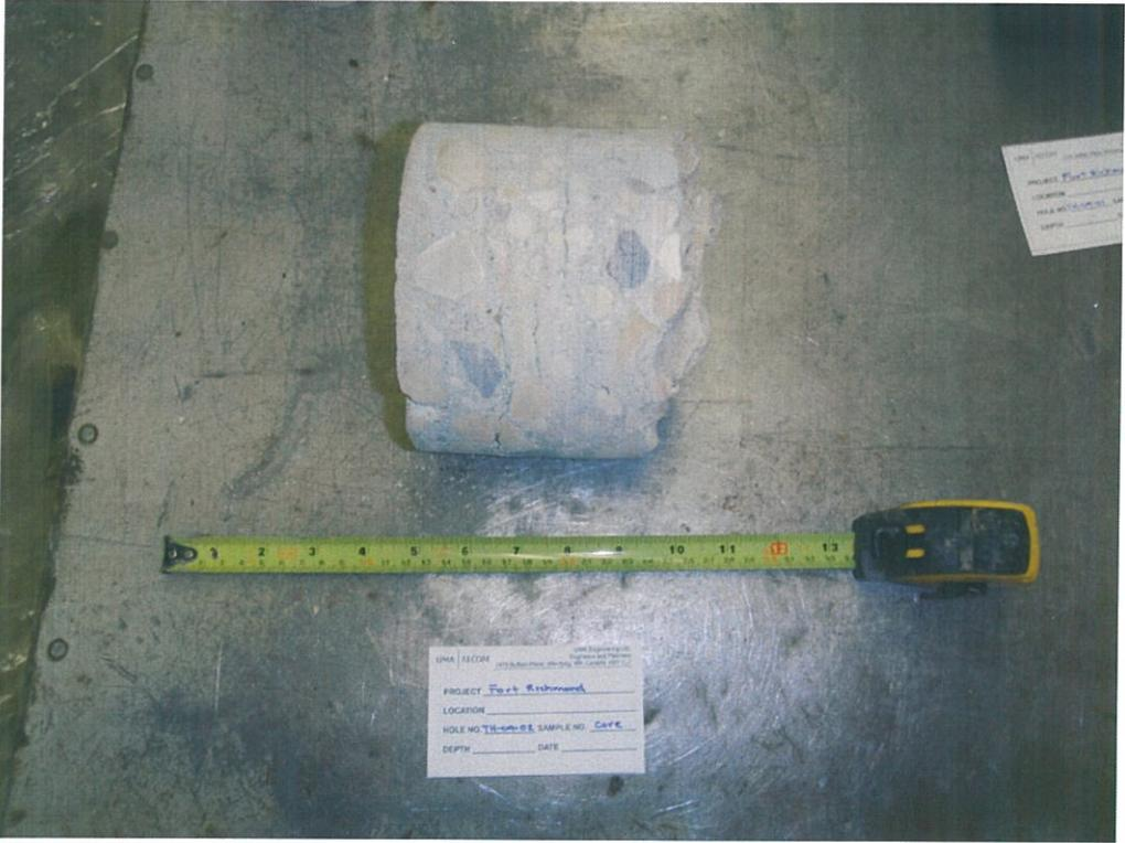
Photo 2: Concrete core sample from TH-09-02
