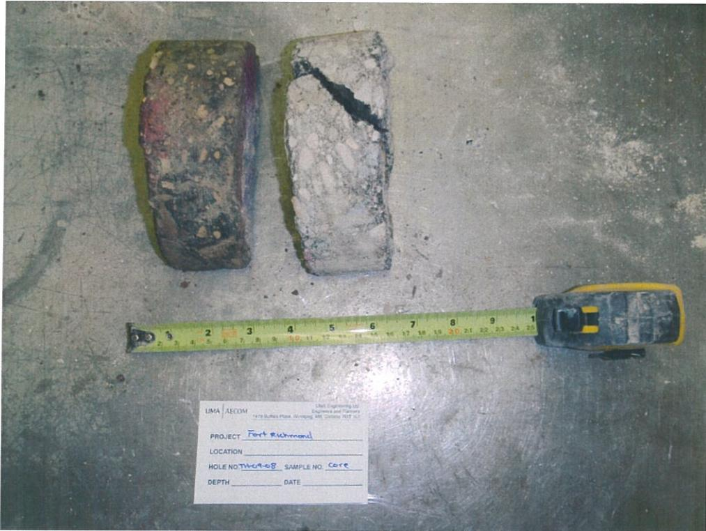
Photo 9: Asphalt core sample from TH-09-08
