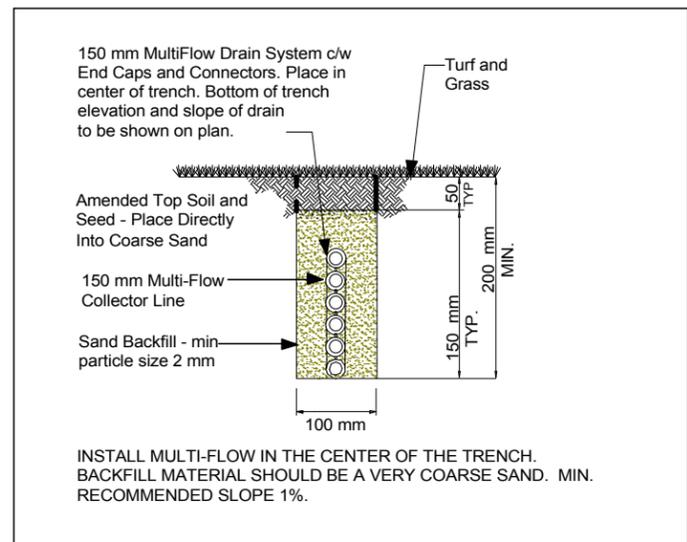
**MULTI-FLOW DRAIN IN TURF AND GRASS DETAIL (D5)**
