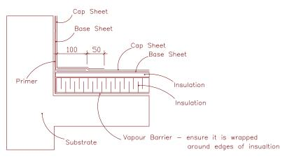
Note: Modified Bitumen stipping used in conjunction with 4 ply felt membrane is to have base sheet extend 12" onto flat and cap sheet 18" onto flat.
