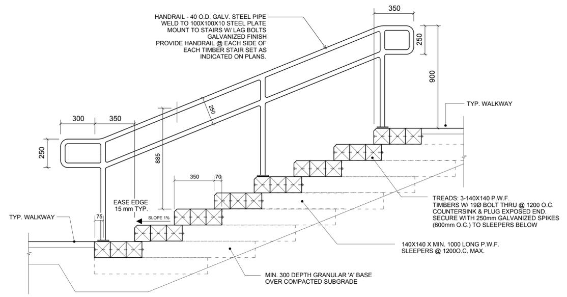
5 TIMBER STAIR AND RAILING SECTION 1:15 (REVISE TO SUIT # OF RISERS)
