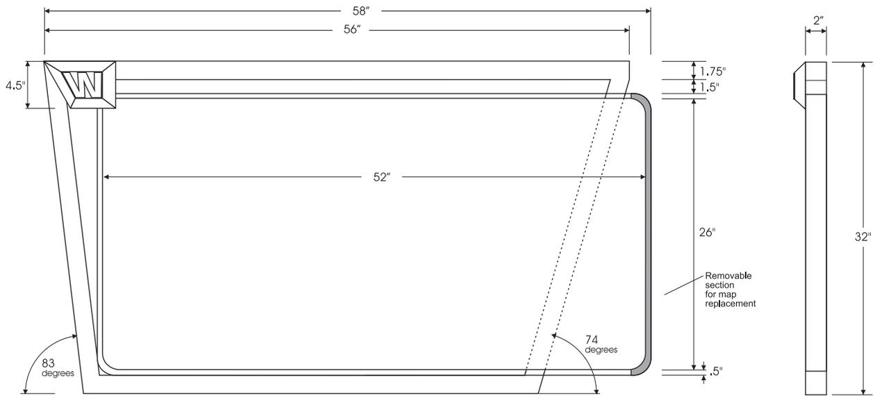
MDF material or equivalent, painted to match. Attached to frame with VHB tape. See details drawing No. 7.
