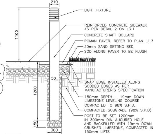
**10 BOLLARD SIDEWALK LIGHTING INSTALLATION DETAIL**
