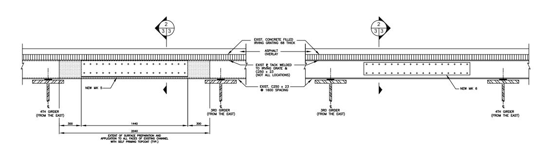
**ELEVATION - DECK CHANNEL REINFORCEMENT** BETWEEN GIRDERS 3 & 4 (TYPE 3 REPAIR)
