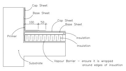
Note: Modified Bitumen stipping used in conjunction with 4 ply felt membrane is to have base sheet extend 12" onto flat and cap sheet 18" onto flat.
