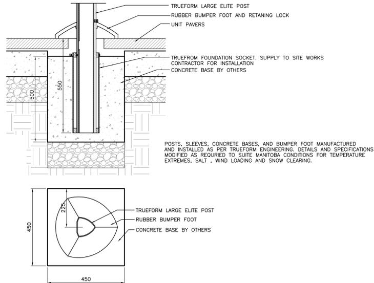
DETAIL 3 - ELITE POLE FOUNDATION SOCKET IN CONCRETE BASE
