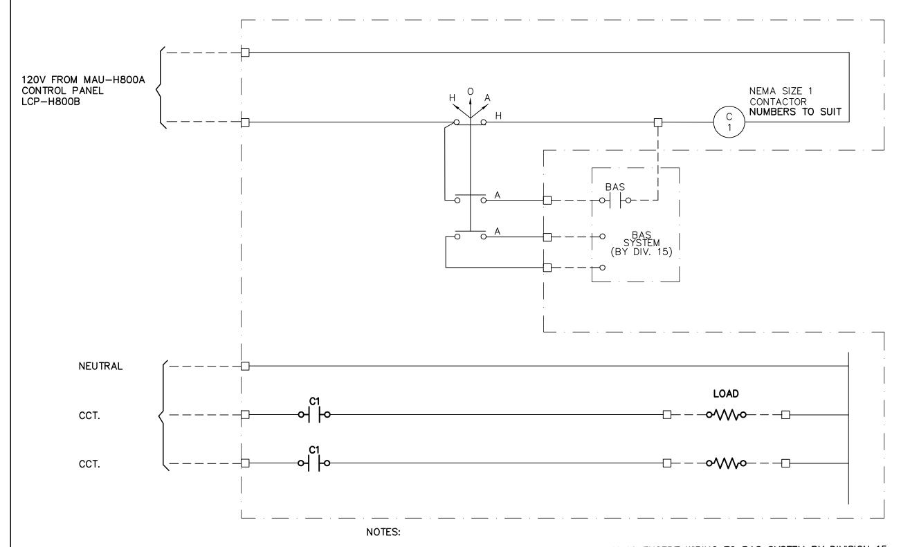
1. LCP-H800A AND ALL FIELD WIRING BY DIVISION 16 EXCEPT WIRING TO BAS SYSTEM BY DIVISION 15.
