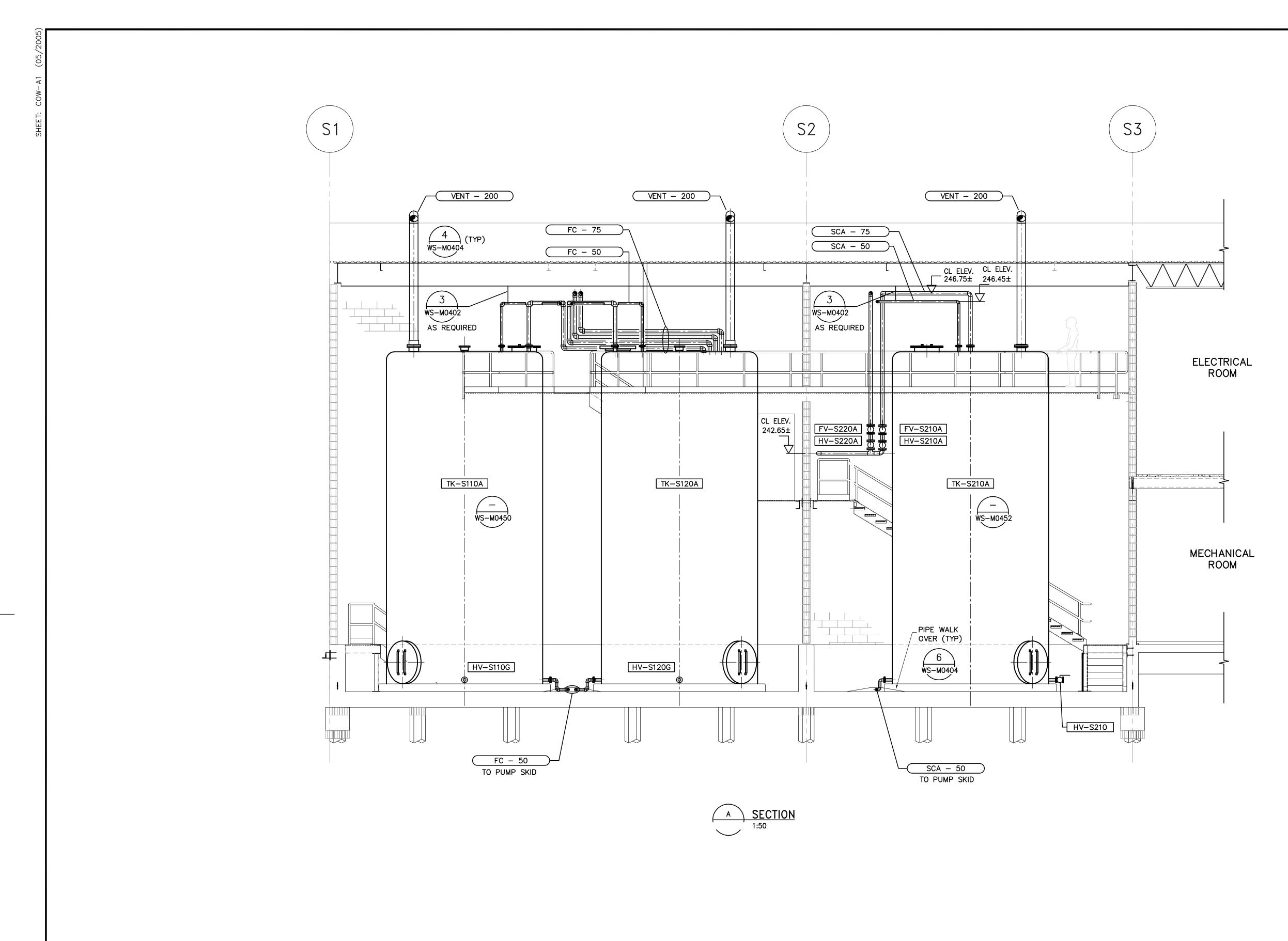
NOTE: 1. SLOPE FILL LINES TO TANKS. 2. SEE DRAWINGS WS-M0450 AND WS-M0452 FOR TANK DETAILS AND NOZZLE SCHEDULE.
