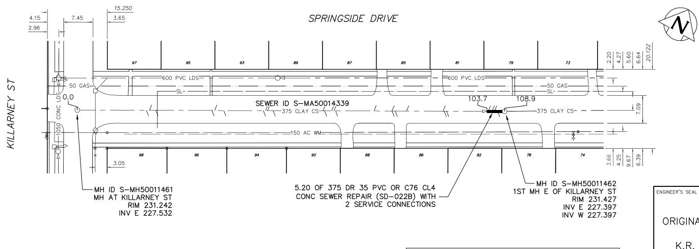
SEWER JUNCTION INFORMATION FROM SEWER VIDEO INSPECTION S-MA50014339 DISTANCE FROM MH ID S-MH50011461 104.70 E 150ø NORTH 105.70 E NORTH 106.30 E 150ø NORTH 107.10 E SOUTH
