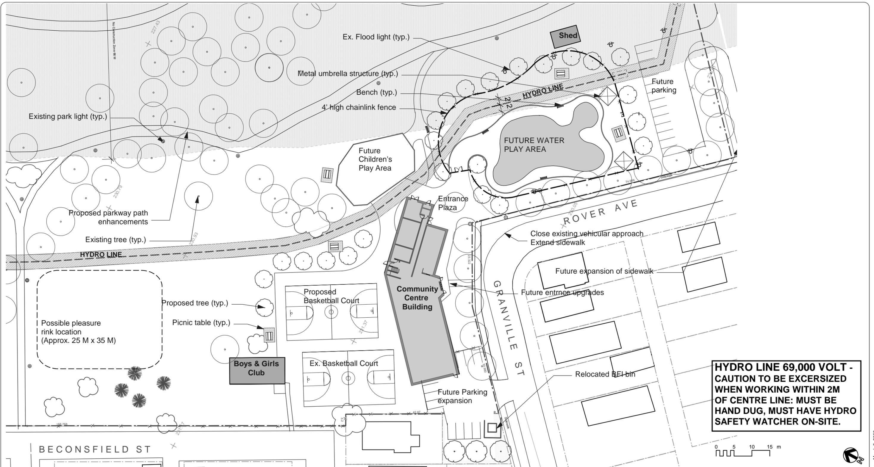
**HYDRO LINE 69,000 VOLT - CAUTION TO BE EXERCISED WHEN WORKING WITHIN 2M OF CENTRE LINE: MUST BE HAND DUG, MUST HAVE HYDRO SAFETY WATCHER ON-SITE.**
