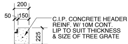
**DETAIL 'B' CONC. HEADER SECTION**
