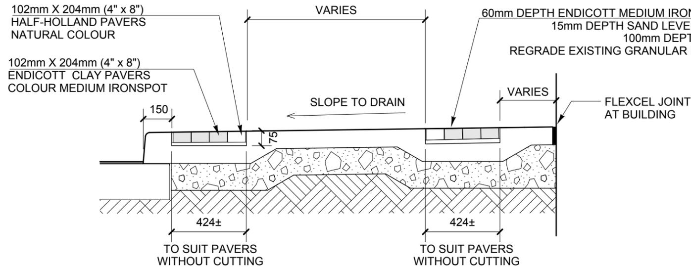
**1 CONCRETE WALKWAY PAVING SECTION**
