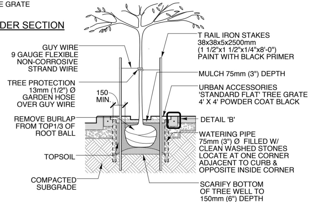
**SECTION A-A TREE WELL CONSTRUCTION & PLANTING**
