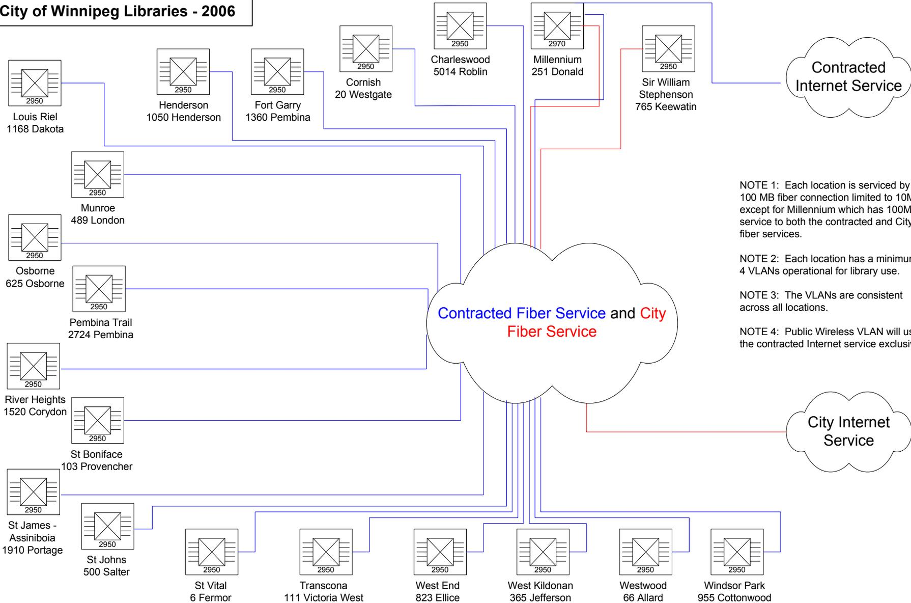
NOTE 1: Each location is serviced by a 100 MB fiber connection limited to 10MB except for Millennium which has 100MB service to both the contracted and City fiber services.
