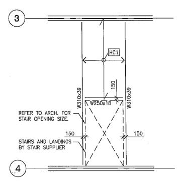
Provide steel beams around the Main Floor stair opening as shown. Provide 125mm wide pocket in concrete walls for beam bearing.
