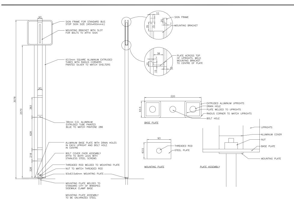
ALL DIMENSIONS PROVIDED FOR INFORMATION ON DESIGN INTENT. BIDDER TO SUPPLY DETAILED SHOP DRAWINGS WITH TENDER SUBMISSION FOR ALL ITEMS. DRAWINGS TO INCLUDE ALL MATERIALS, CONSTRUCTION TECHNIQUES, DIMENSIONS, FITTINGS, FASTENINGS, CONNECTION DETAILS, ELECTRICAL REQUIREMENTS, LIGHTING, ETC.
