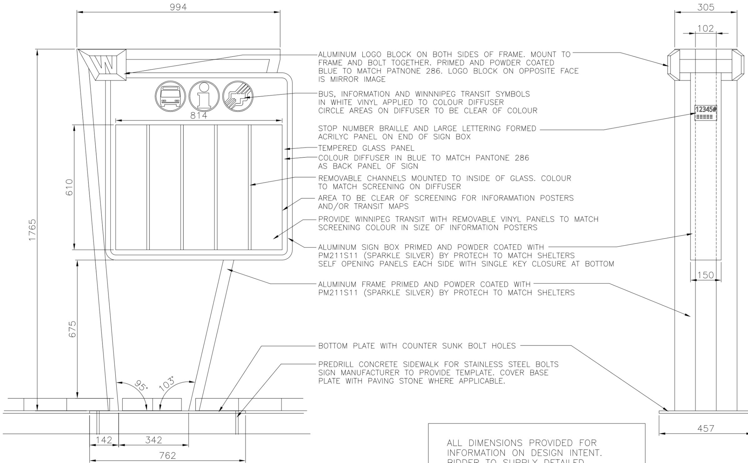
ALUMINUM LOGO BLOCK ON BOTH SIDES OF FRAME. MOUNT TO FRAME AND BOLT TOGETHER. PRIMED AND POWDER COATED BLUE TO MATCH PATNONE 286. LOGO BLOCK ON OPPOSITE FACE IS MIRROR IMAGE
