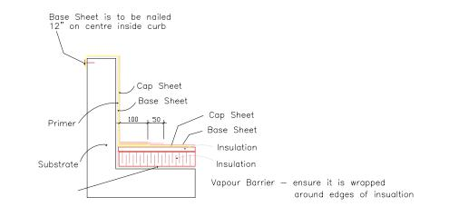
Note: Details are to be similar for inverted roof assemblies
