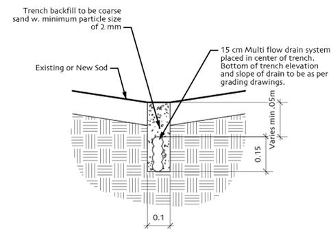
4 Multi-Flow Drain in Turf Area
