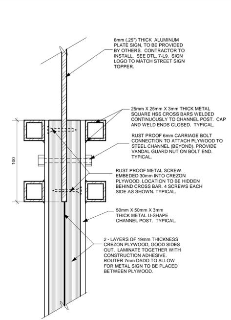
7 SIGN CONNECTION DETAIL SECTION "A"
