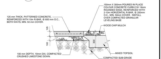
10 SHRUB BED/CONCRETE PAVING SECTION
