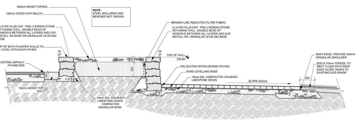
4 PLANTER WALL/INTERLOCKING PAVING SECTION
