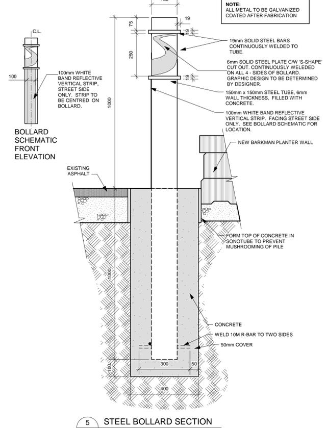
5 STEEL BOLLARD SECTION
