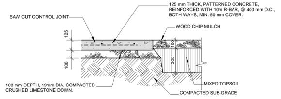
6 SHRUB BED / CONCRETE PAVING SECTION
