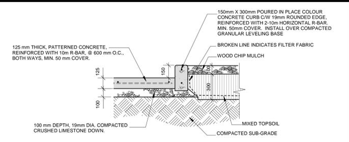
4 SHRUB BED / CONCRETE PAVING SECTION
