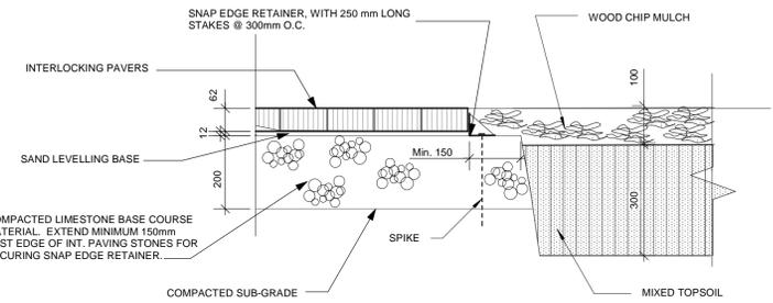
7 INTERLOCKING PAVING EDGE SECTION BY GRASS
