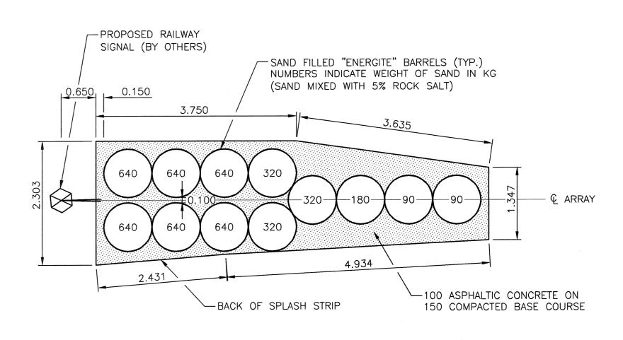
DETAIL 'B' SCALE 1:50 DESIGN SPEED = 80 KPH
