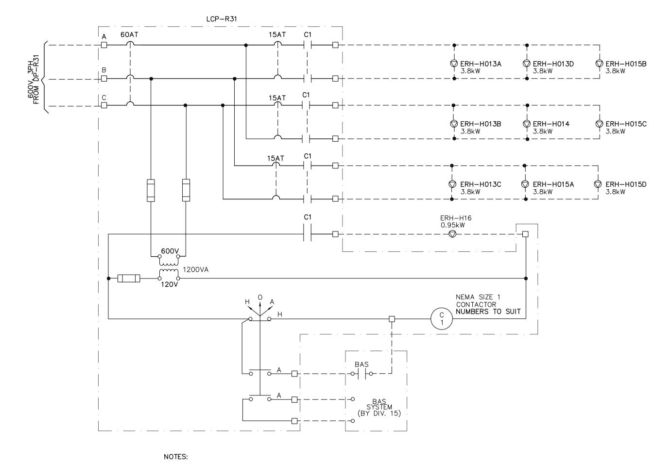
1. LCP-R31 AND ALL FIELD WIRING BY DIVISION 16 EXCEPT WIRING TO BAS SYSTEM BY DIVISION 15.
