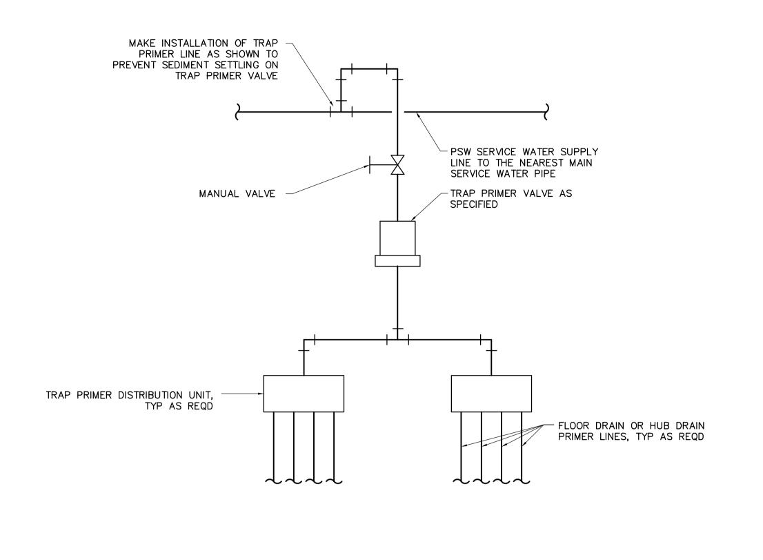
FLOOR DRAIN TRAP PRIMER DETAIL
